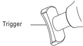
The rotation speed of drill saw can be controlled by how hard the trigger is squeezed. Squeeze the trigger fully for the fastest speed and squeeze it lightly for the slowest
