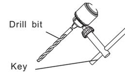
Twist the key, clockwise to clamp drill chuck and counter clockwise to loosen drill chuck
